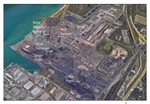
The plant's 7 million metric tons of annual CO2e<sup>1</sup> emissions are scattered across a vast, complex operation shown in the picture. They come from large and small sources, including blast furnaces, coke ovens, boilers, sinter plant operations, basic oxygen furnaces, and flares.
